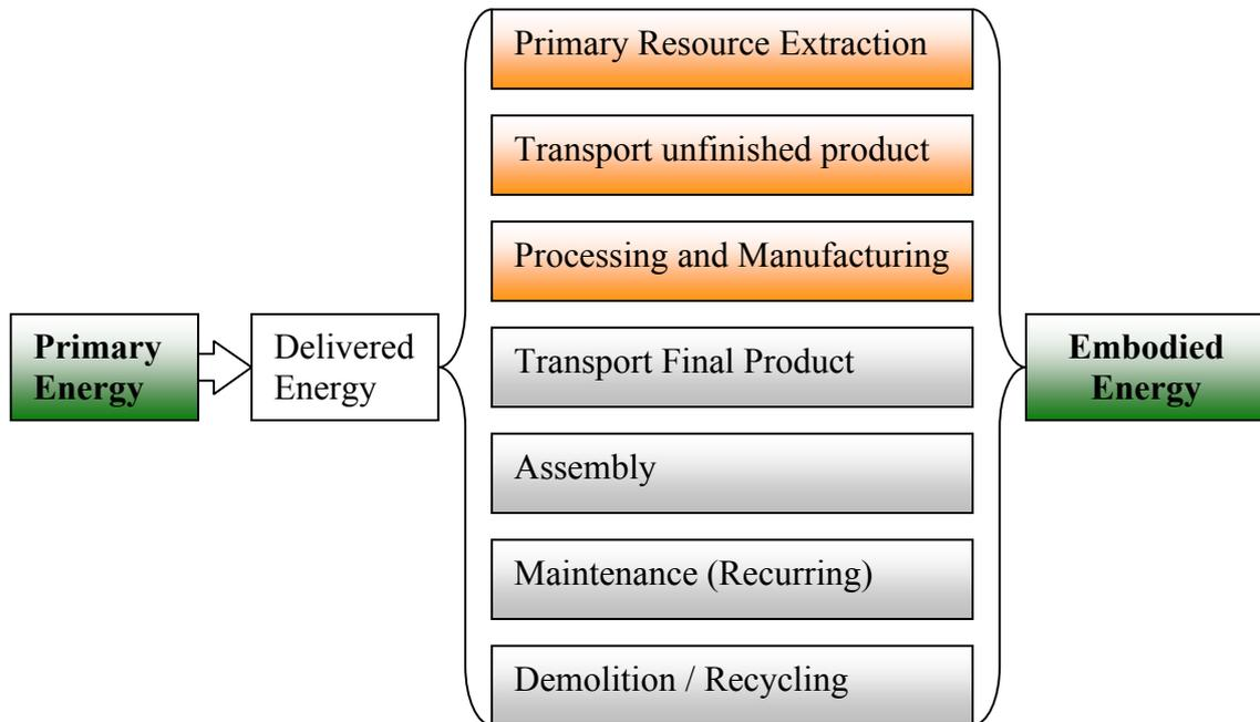
**Figure 1: Breakdown of embodied energy calculations. Most embodied energy figures for specific materials are quoted using a “cradle to gate” boundary (includes orange boxes). Consumers must also consider transport, assembly, maintenance and demolition components of embodied energy. In addition, care should be taken to ensure that primary energy consumption is calculated, not delivered energy (which will understate the real energy cost).**
